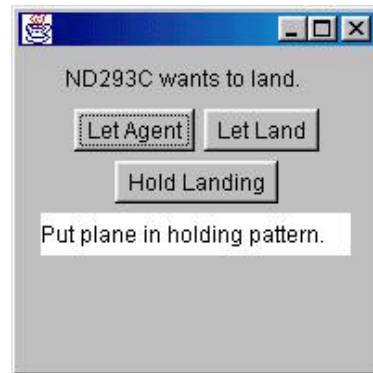
Figure 3. Landing dialog window. “Let Agent” allows the agent to take care of the landing. “Let Land” is used by the human operator to give permission to land. “Hold Landing” is used by the human operator to decline clearance for landing and to send the plane into holding pattern. The agent action is shown in the bottom of display.
