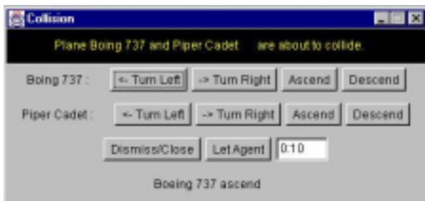
Figure 2. The collision dialog window. Each plane can receive different commands: Turn left or right, ascend or descend. “Dismiss/Close” button will do nothing to the planes, whereas “Let Agent” button will allow the agent to perform the actions being suggested by the agent at the bottom of the screen. When the timer (10 seconds is shown) runs out, the agent will perform the suggested action.
