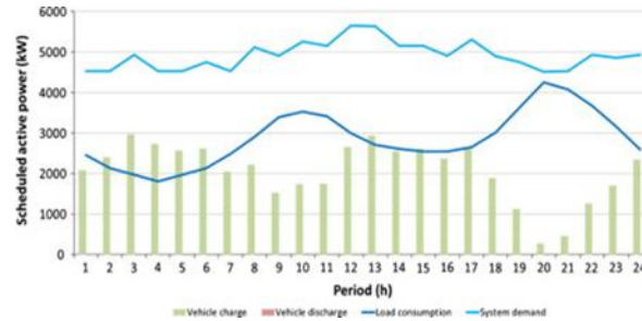
Figure 5: Power Demand Curve
