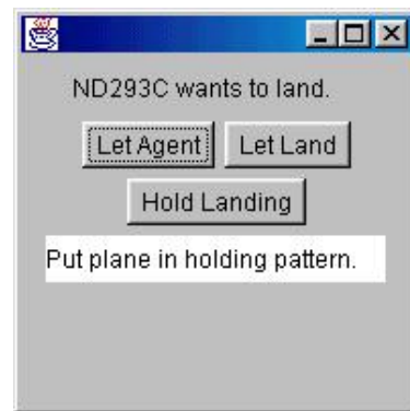
Figure 5. Landing dialog window. “Let Agent” allows the agent to take care of the landing. “Let Land” is used by the human operator to give permission to land. “Hold Landing” is used by the human operator to decline clearance for landing and to send the plane into holding pattern. The agent action is shown in the bottom of display.
